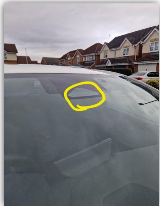
Front facing Camera, Light Sensor and Rain Sensor
