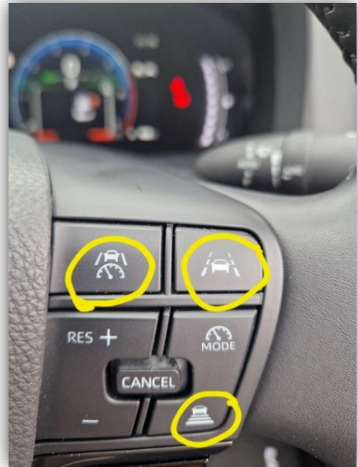
Adaptive Cruise Control with Speed and Distance
