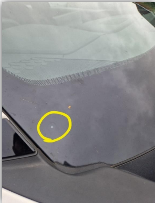
One of the two side cameras used for exit assistance
